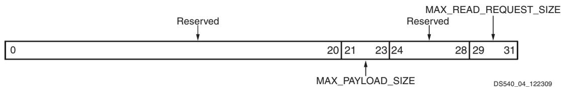
Figure 4: PCIe Request Control Register
