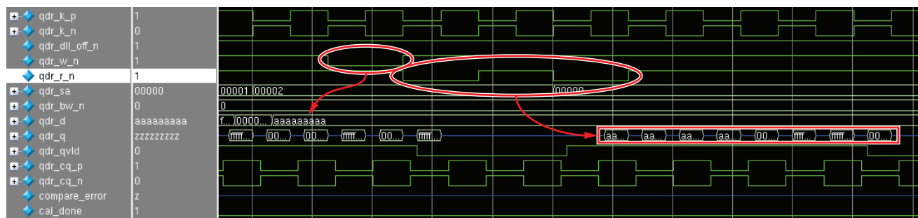
Figure 2-48: Write and Read for Second Stage Read Calibration
