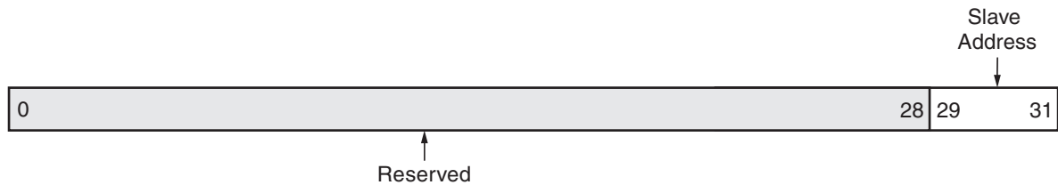
Figure 11: Ten Bit Address Register (TEN_ADR)
