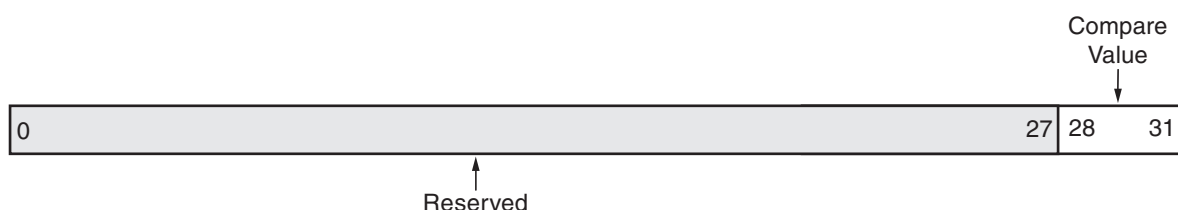
Figure 14: Receive FIFO Programmable Depth Interrupt Register (Rc_FIFO_PIRQ)
