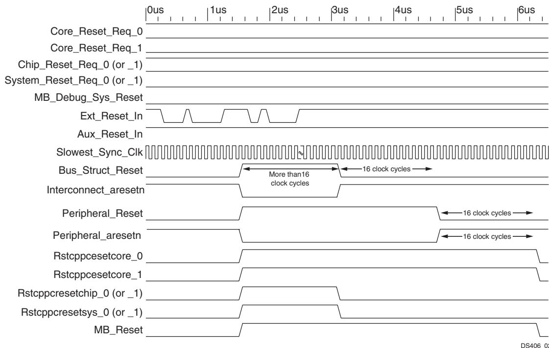
*Figure 2: Processor System Reset Module - Ext\_Reset\_In (active low)*
