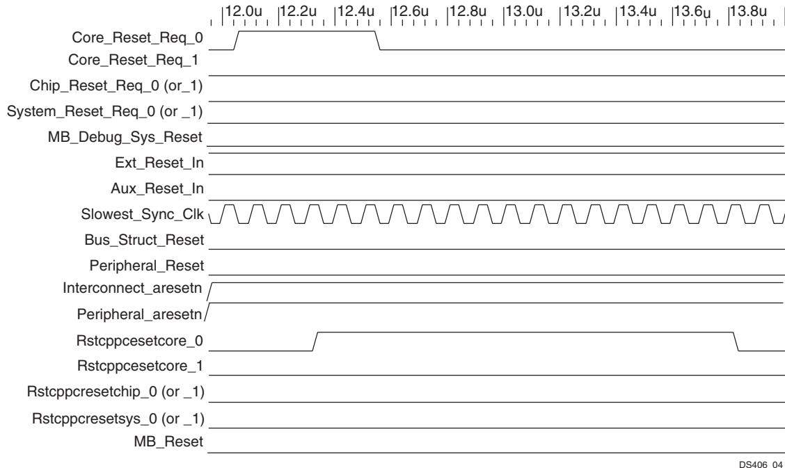
Figure 4: Processor System Reset Module - Core\_Reset\_Req
