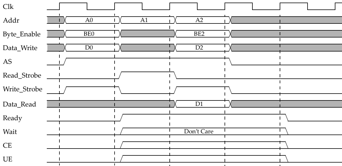
Figure 2-8: Back-to-Back Mixed Write/Read Operation, 0 Wait States
