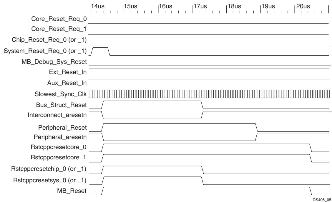
Figure 5: Processor System Reset Module - System\_Reset\_Req
